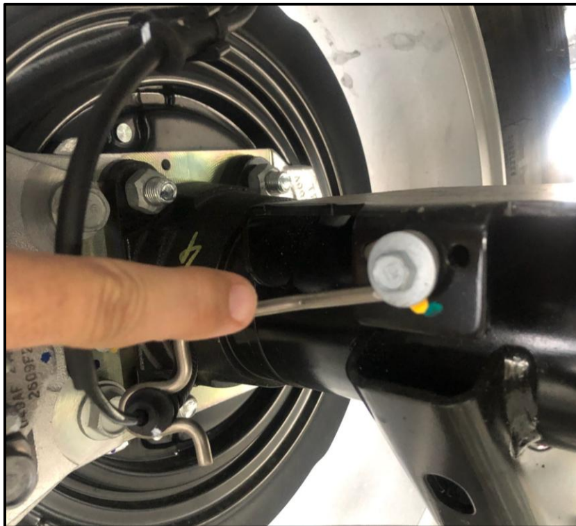
Brake Line Wire Form to be removed
