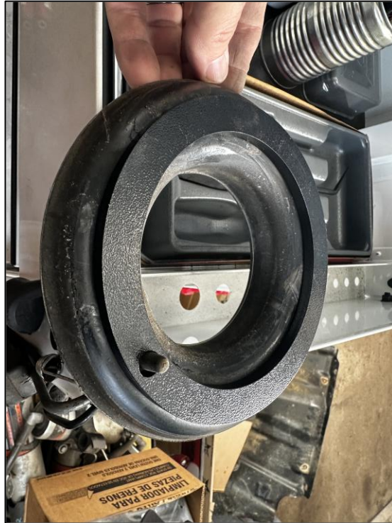
Top lean Correction Seat on Top of OEM Upper Spring Seat
