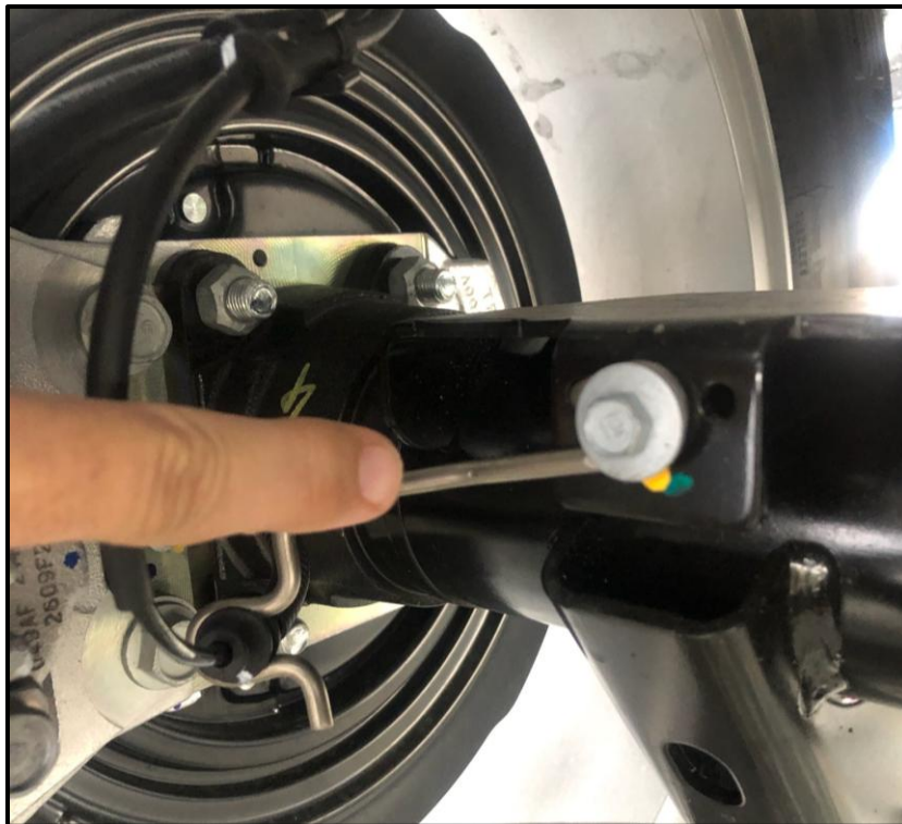
Brake Line Wire Form to be removed
