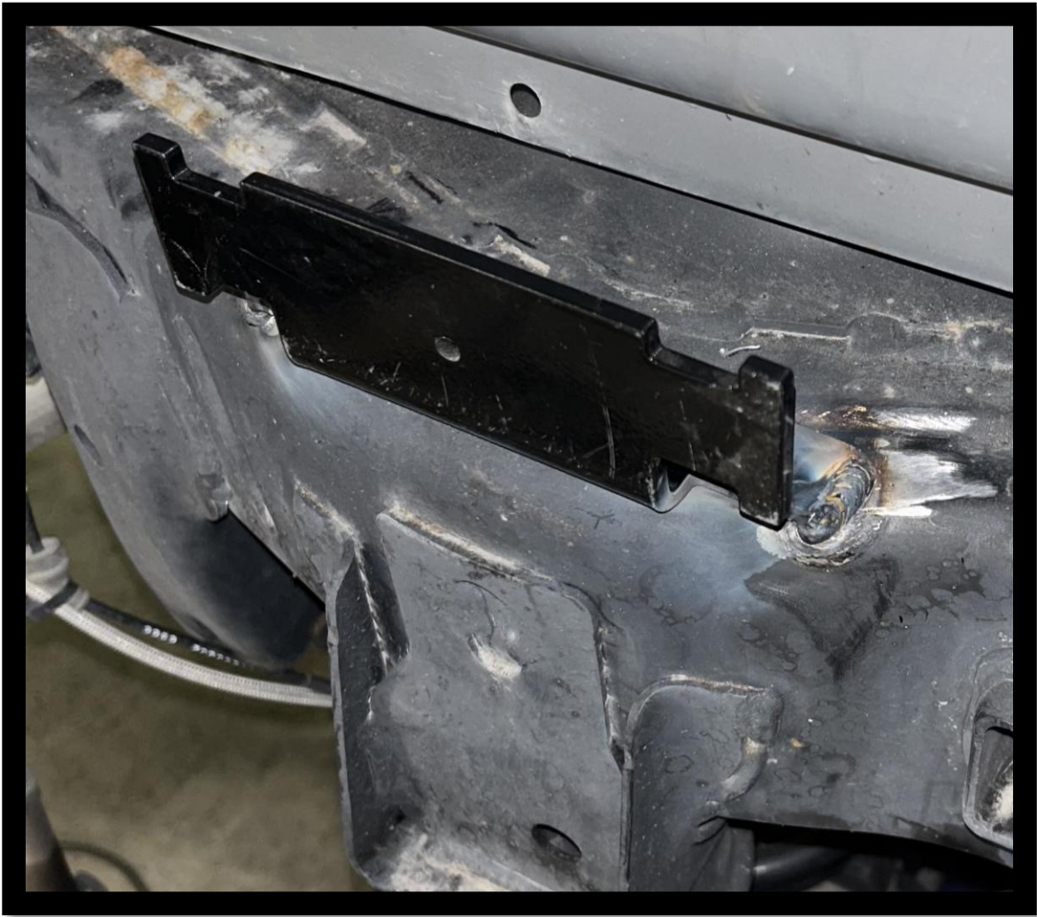
Ressy Mount Welded to the Frame
