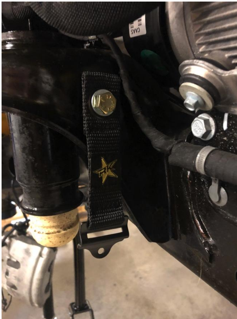
Sway bar strap retainer installed
