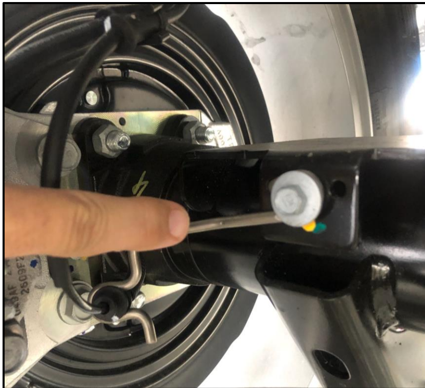
Brake Line Wire Form to be removed
