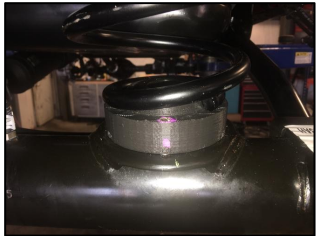
Pass. Side Spring Seat Installed with Coil
