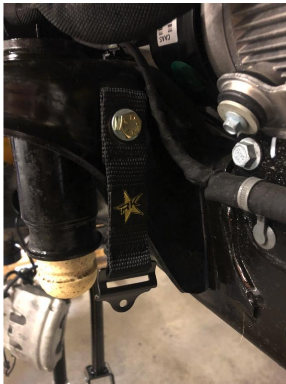
Sway bar strap retainer installed
