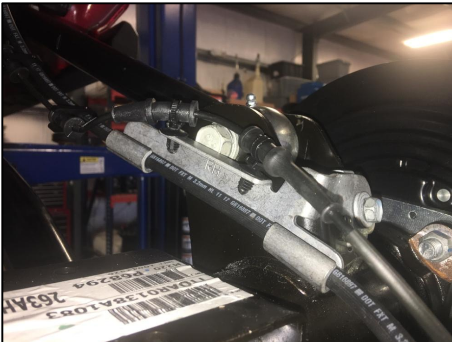
New Orientation for Rear Brake Line Brackets
