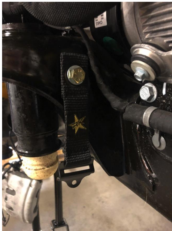
Sway bar strap retainer installed
