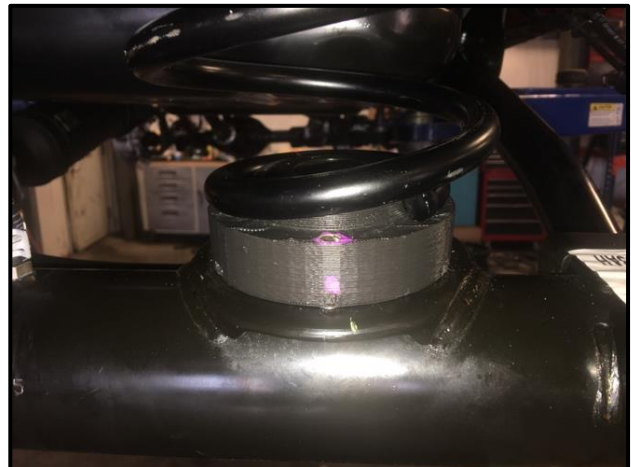
Pass. Side Spring Seat Installed with Coil
