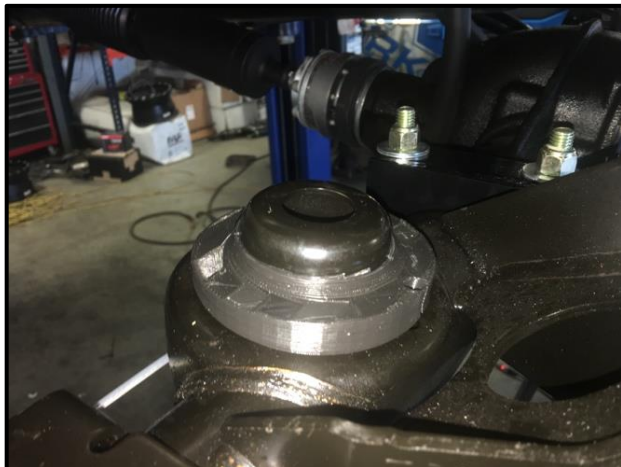
Driver Side Spring Seat Installed
