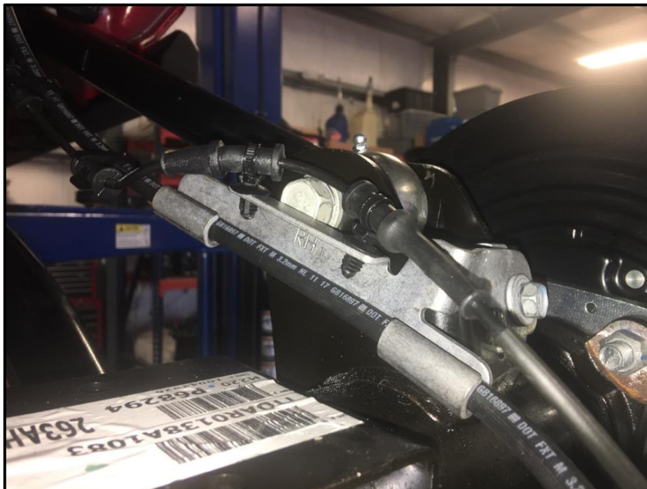
New Orientation for Rear Brake Line Brackets
