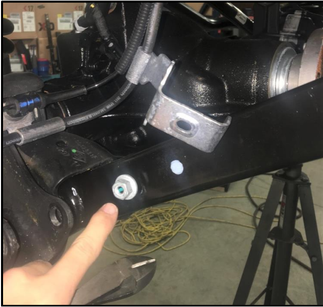
Remove Brake Lines from Arms
