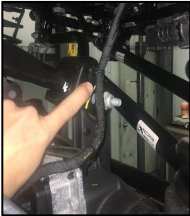
Remove Brake Lines from Arms
