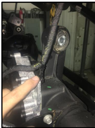
Remove Brake Lines from Arms
