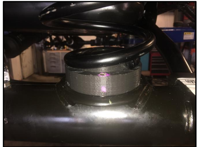
Pass. Side Spring Seat Installed with Coil
