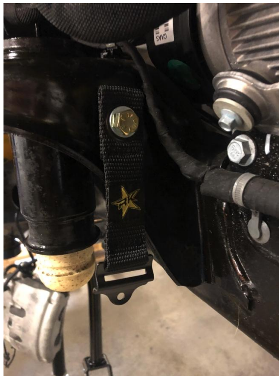
Sway bar strap retainer installed
