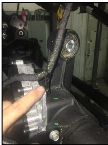
Remove Brake Lines from Arms
