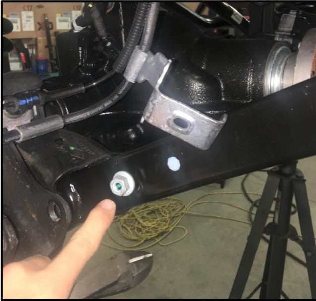
Remove Brake Lines from Arms
