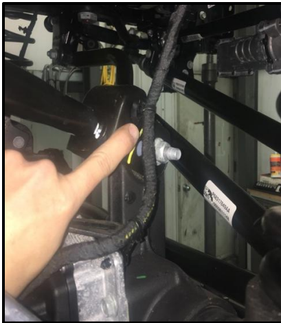
Remove Brake Lines from Arms
