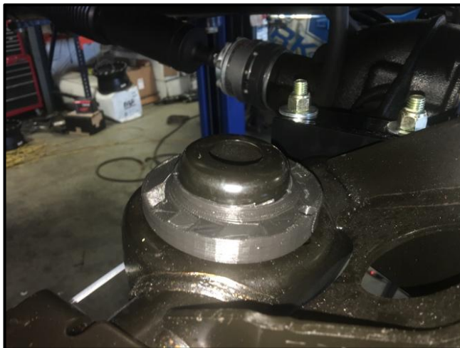
Driver Side Spring Seat Installed
