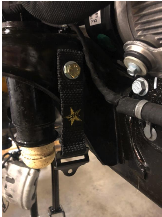
Sway bar strap retainer installed
