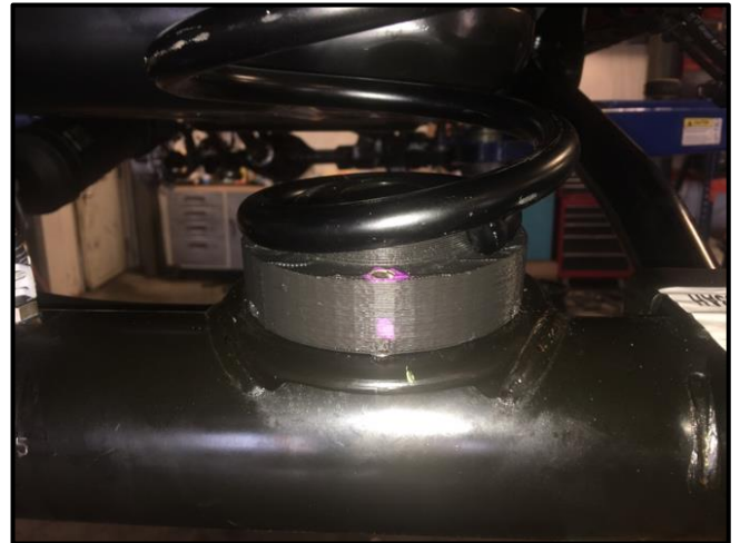
Pass. Side Spring Seat Installed with Coil
