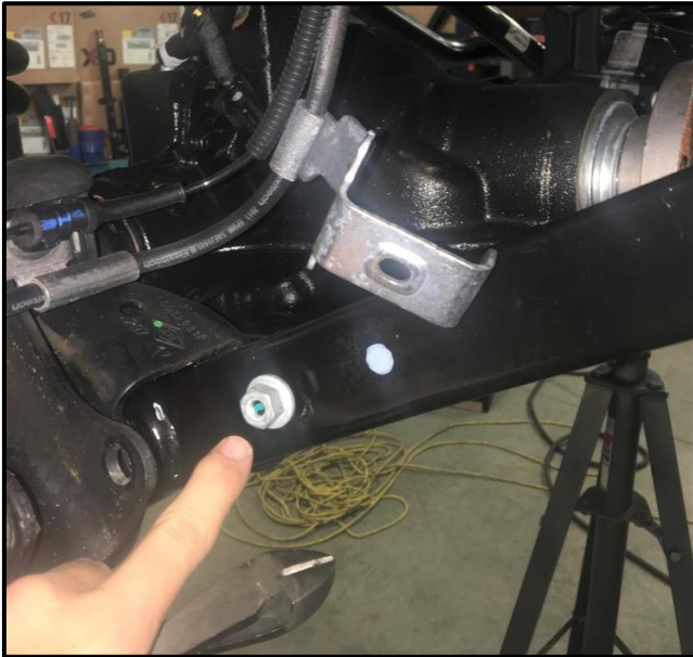
Remove Brake Lines from Arms
