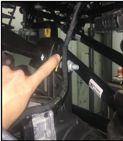
Remove Brake Lines from Arms
