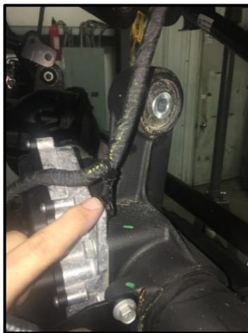
Remove Brake Lines from Arms
