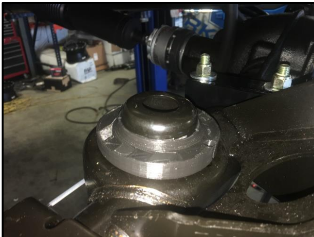
Driver Side Spring Seat Installed
