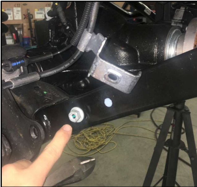
Remove Brake Lines from Arms
