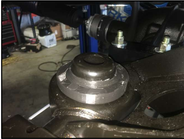
Driver Side Spring Seat Installed
