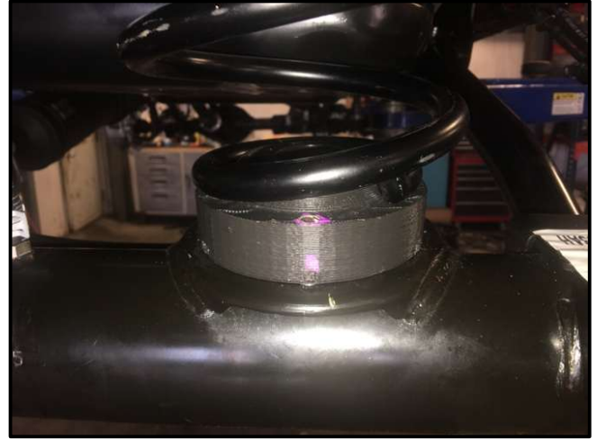
Pass. Side Spring Seat Installed with Coil
