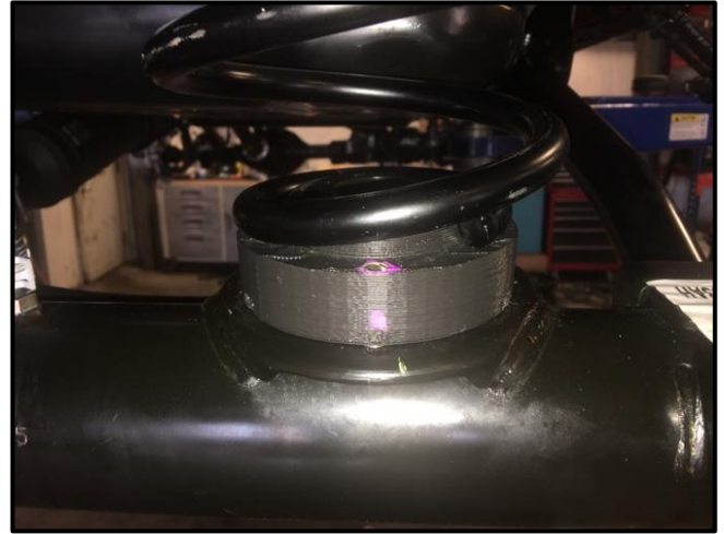
Pass. Side Spring Seat Installed with Coil
