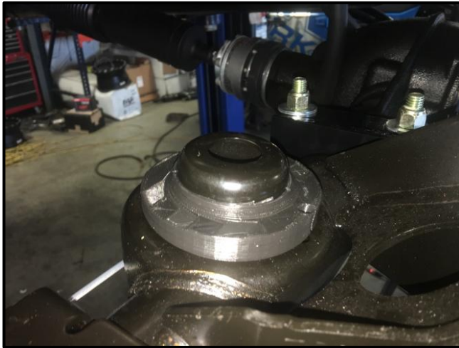
Driver Side Spring Seat Installed
