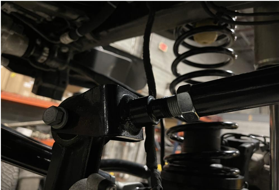
Pass. Side Front Upper Showing Clevis Adjuster at the Axle Connection.
