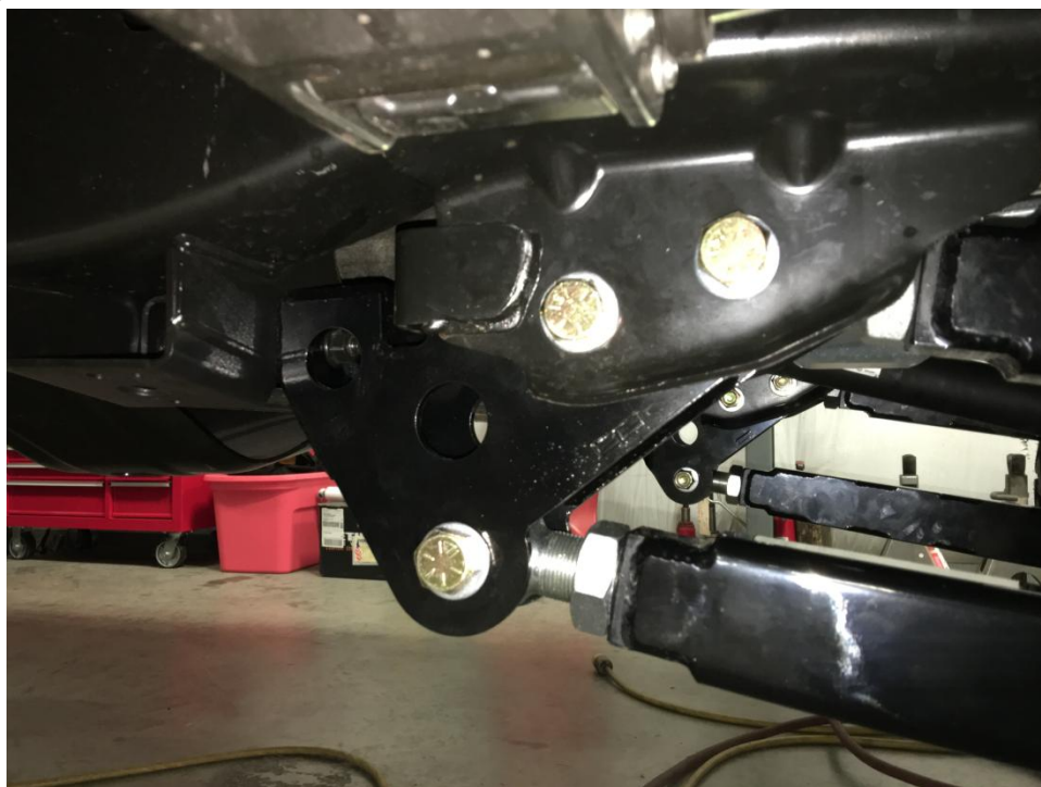
4 Link Long Arm Mounts, 2017-2022 Model Shown
