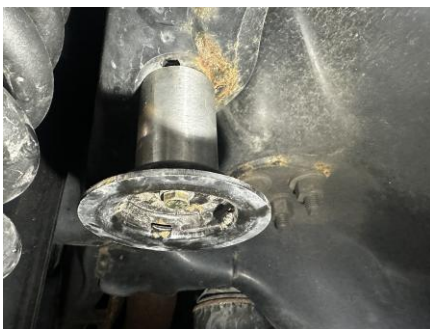
Billet Bump Stop Extension Installed
