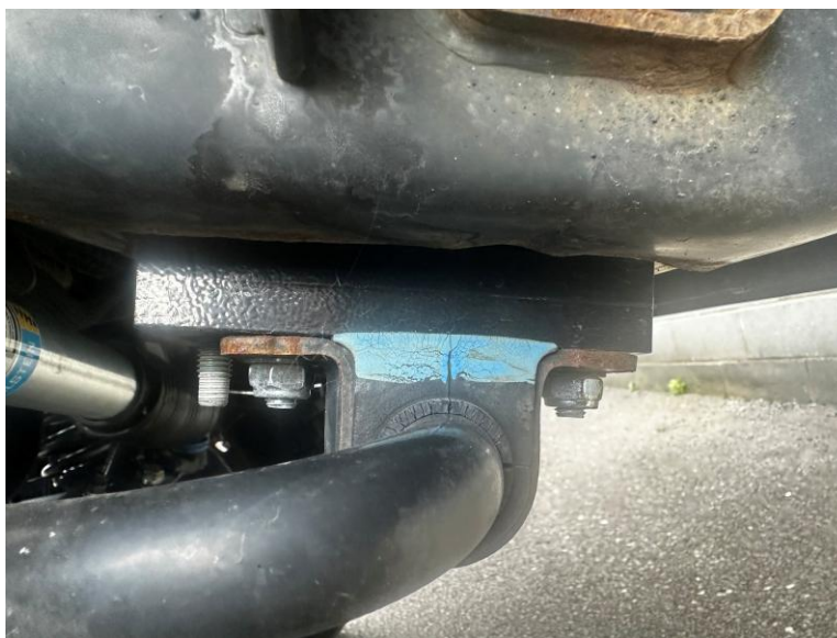
PB+J Sway Bar Link Relocation Block Installed
