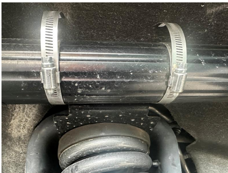
Front Rassy Mount Under the Coil Spring Isolator
