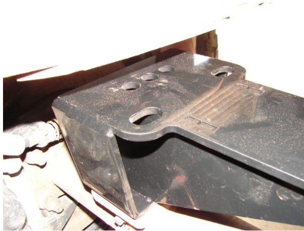
Fabbed Block w/ Multiple Centering Pins to Center the Rear Axle
