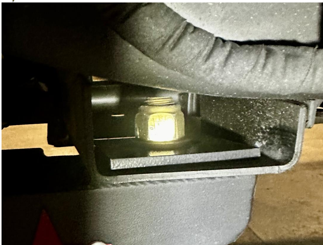
2023 – Present Doubler Plate Inside the Cross Member Shown
