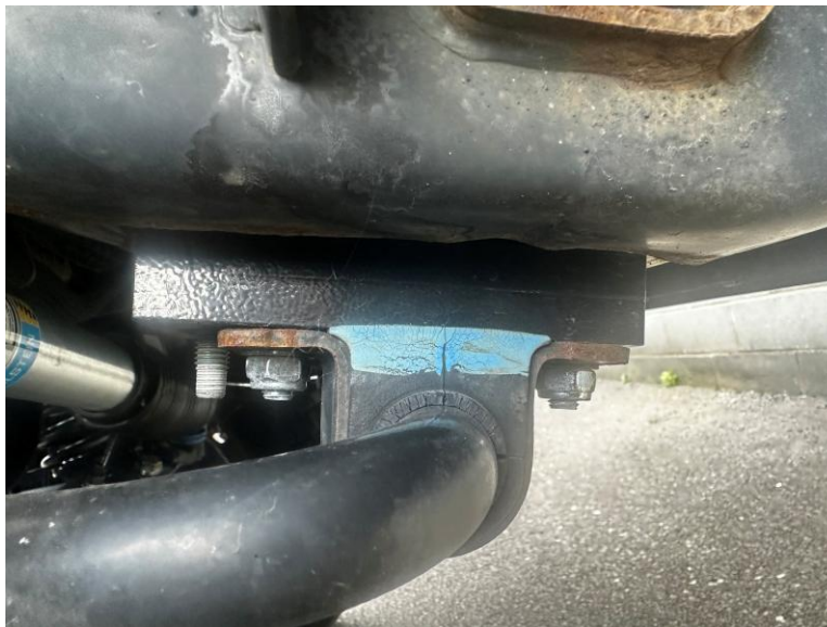
PB+J Sway Bar Link Relocation Block Installed
