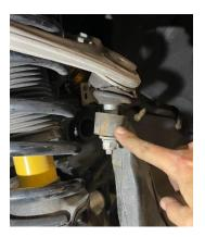
10) Remove the upper sway bar link. (Shown on right)
