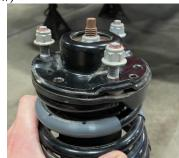
16) Insert the supplied 10mm bolts into bottom of spacer into the recessed slots. These are designed to capture the bolt head when installed on top of strut. Pics attached.
